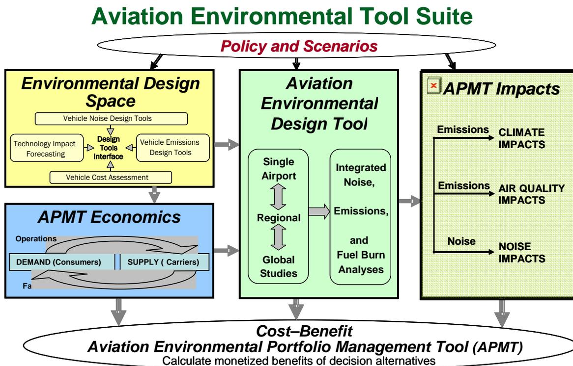
**FIGURE 1** Simplified schematic of the FAA Office of Environment and Energy’s integrated tools suite currently under development, consisting of the Environmental Design Space, Aviation Environmental Portfolio Management Tool, and Aviation Environmental Design Tool.
